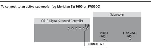
The Meridian SW1600 and SW5500 subwoofers provide both digital and analogue inputs, allowing you to connect them to either the digital or analogue subwoofer outputs of the G61R. The analogue connection must be used if you do not have a digital main speaker.
