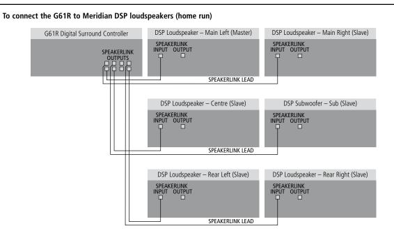
This is an alternative to the "daisy chain" wiring configuration shown in the previous section.
