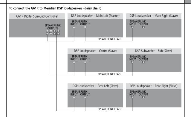
This is an alternative to the "home run" wiring configuration shown in the next section.
