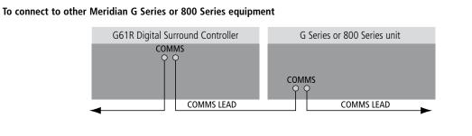
In a system of Meridian products the products should be linked together in a chain, via the COMMS sockets, using the Comms leads supplied with each product. The sequence in which you connect the units is not important.
