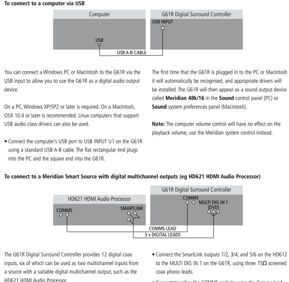
• Connect together the COMMS sockets using the Comms lead provided.
