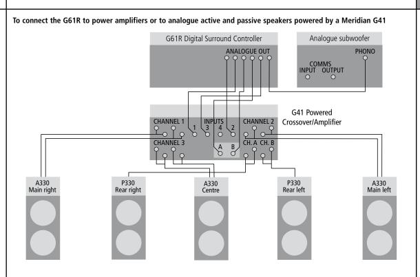
The G61R provides eight analogue outputs to allow you to connect to power amplifiers and passive loudspeakers, or 300 Series Active and Passive Installation Loudspeakers powered by the G41 Active Crossover Amplifier.
